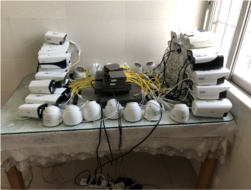
Stability tests with cameras over 30 days in a real environment
