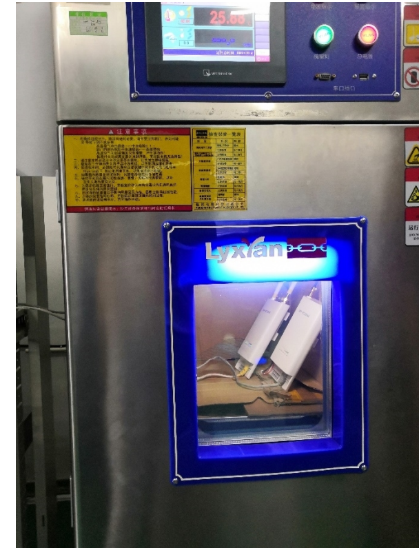
7*24 hours, -30°~+60° temperature cycle aging test
