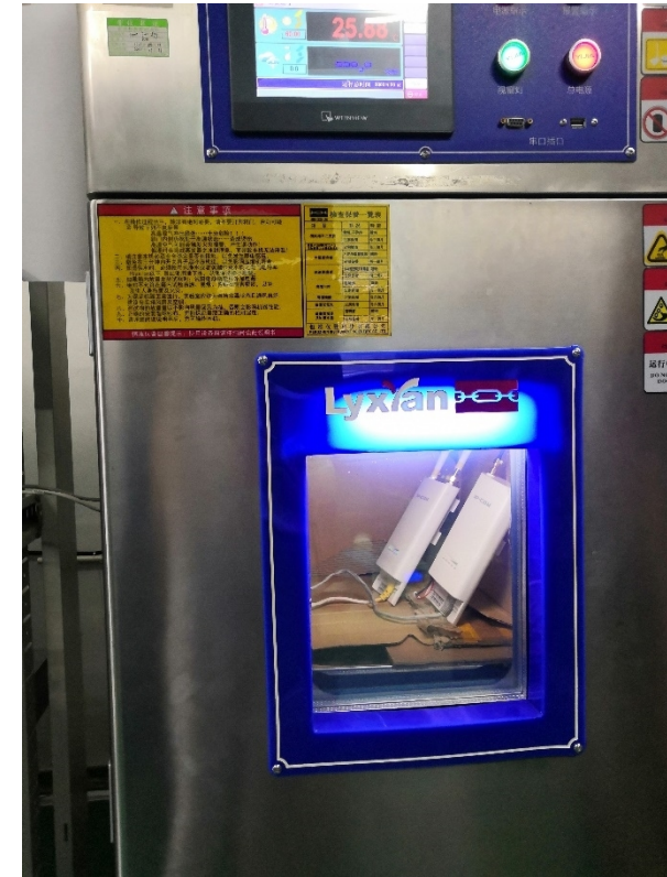
7*24 hours, -30°~+60° temperature cycle aging test
