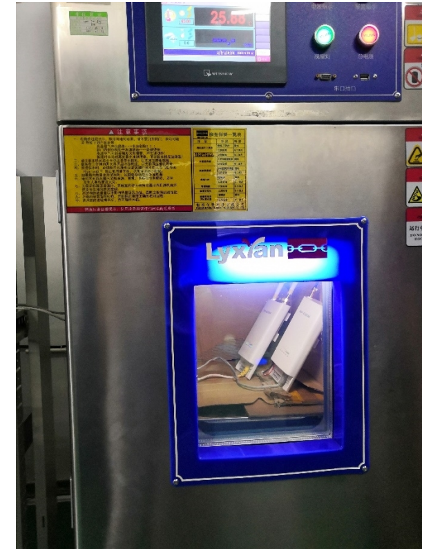
7*24 hours, -30°~+60° temperature cycle aging test
